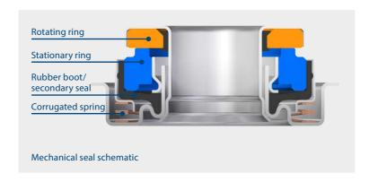
> The secondary seals (rubber boot) are made of a high-performance elastomer HNBR material which offers superb temperature and weather resistance.
